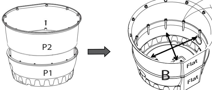
**4)** Connect A and B with screws
